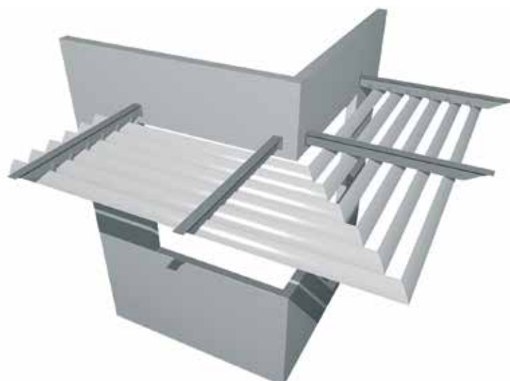
OVERHEAD (HORIZONTAL) BRACKET FIXED LOUVRES WITH CORNER MITRES
