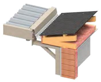
FREE STANDING POST SUPPORTS BOX SECTION ABOVE GUTTER, WITH CAP FLASHING INTO GUTTER. USE THIS OPTION WHEN THERE ARE NO OTHER FIXING POINTS AND THE HOUSE CLADDING IS NOT SUITABLE FOR STRUCTURAL FIXING.
