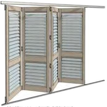
COASTAL 100: 4 PANEL BIFOLDING DOOR WITH 90MM LOUVRE INFILLS
