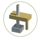
POSTS PROJECTED THROUGH DECK ON TO CONCRETE PAD
