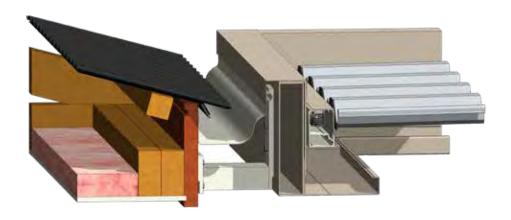
BRACKET FIXED TO FASCIA. BOX SECTION SITS ABOVE GUTTER WITH CAP FLASHING INTO GUTTER.
