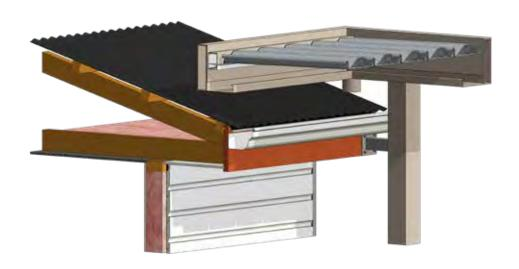
BRACED OR FREE STANDING POST PROJECTS OPENING ROOF OVER HOUSE ROOF.
