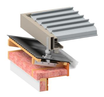
FIXING BRACKET CONNECTED TO RAFTERS AND FLASHED ACCORDINGLY. ROOF IRON OR TILES NEED TO BE LIFTED FOR BRACKET INSTALLATION.
