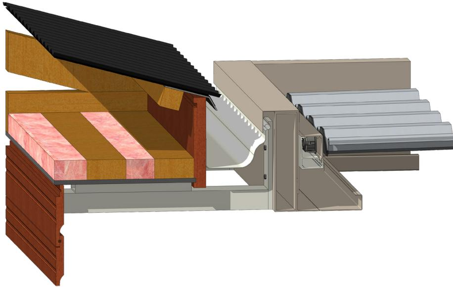
BRACKET FIXED TO UNDERSIDE OF SOFFIT. BOX SECTION SITS ABOVE GUTTER WITH FLASHING INTO GUTTER.
