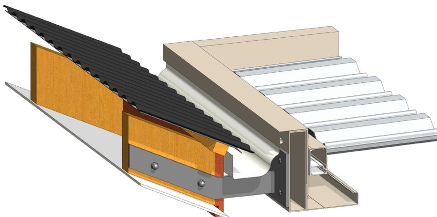
BRACKET FIXED TO RAFTER. BOX SECTION SITS ABOVE GUTTER WITH CAP FLASHING INTO GUTTER.
