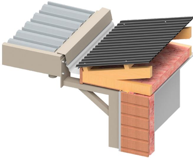
FREE STANDING POST SUPPORTS BOX SECTION ABOVE GUTTER, WITH CAP FLASHING INTO GUTTER.
