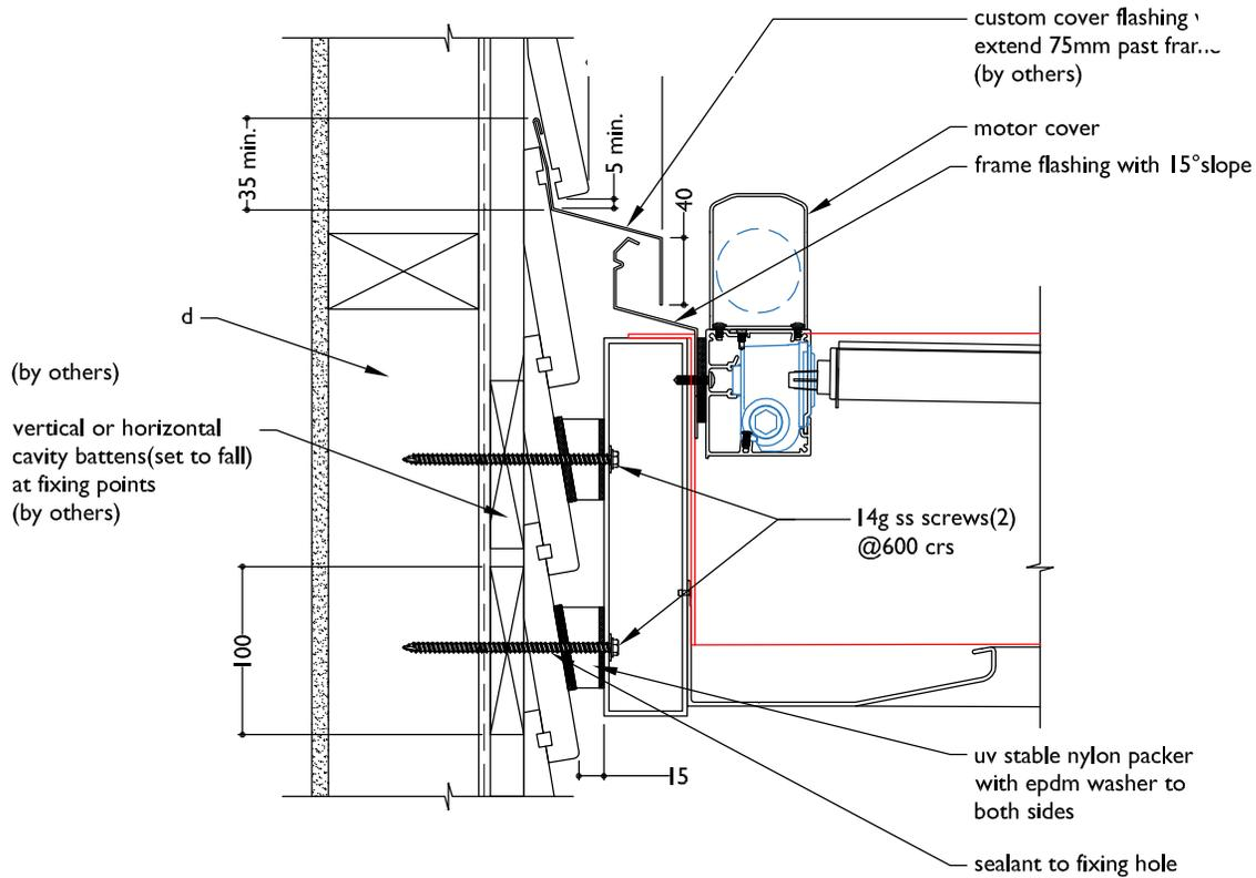
SECTION OPTION 3A - WEATHERBOARD ON TIMBER FRAME
