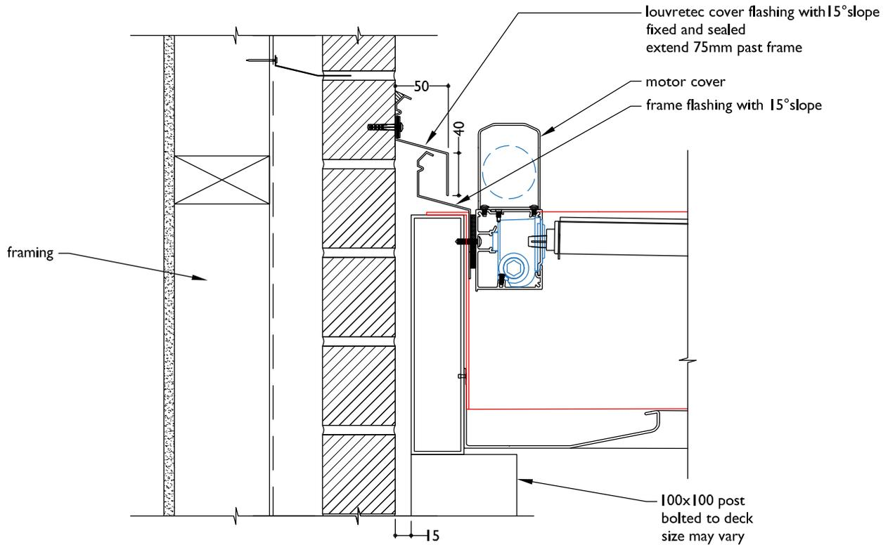
**SECTION COMPOSITE PANEL ON TIMBER FRAME FREE STANDING
