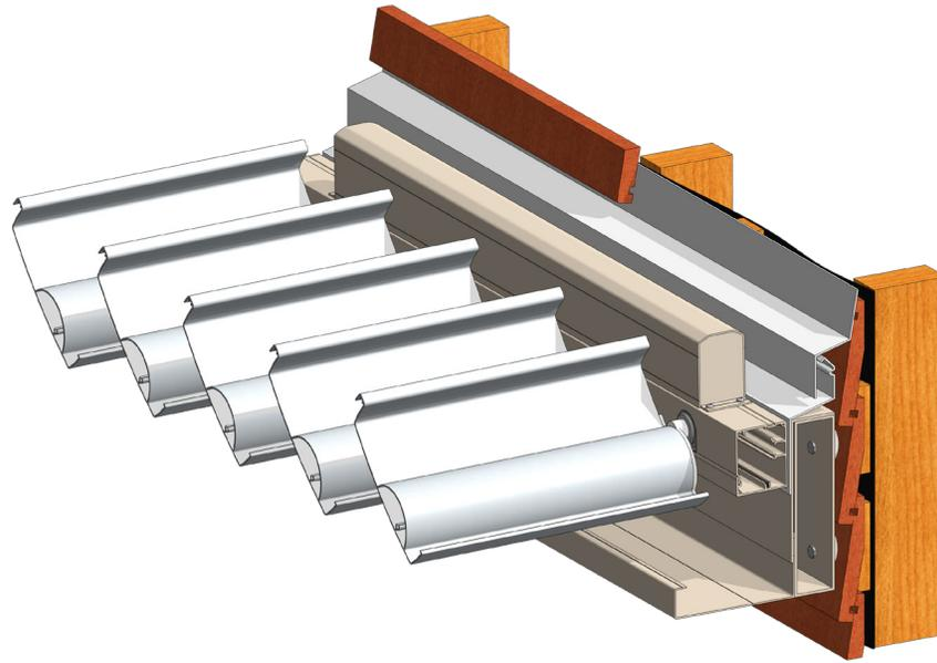
FIXED TO WEATHERBOARD CLADDING ON TIMBER FRAME WITH CAVITY.
