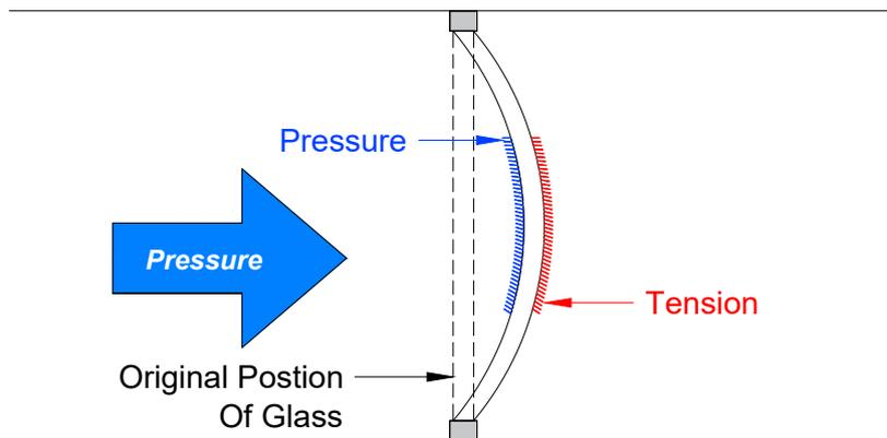
When wind loads are applied to glass it causes both compression and tensile stresses as illustrated in the diagram above.
