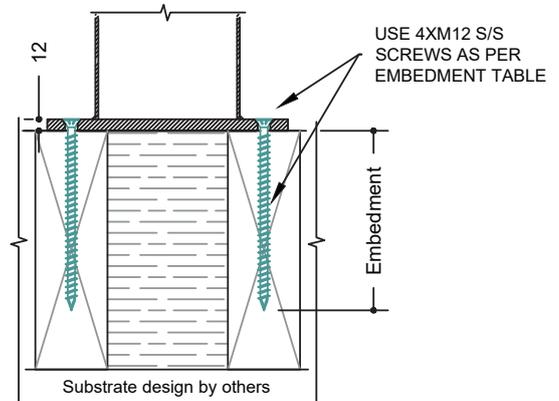
NOTE: ALL POST TO BASE PLATE WELDS MUST BE FULL PENETRATION BUTT WELDS ALL AROUND
